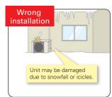
Use a stand to add sufficient height to protect the unit heat exchanger from snow and prevent icicles forming during defrost operation.
